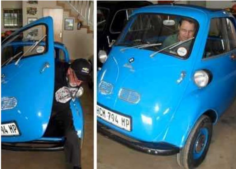
**OPEN DOOR POLICY:** Dave Fall enters and leaves the BMW Isetta through its front-facing door as the steering wheel and instruments swing out of the way. Could it make a comeback?
